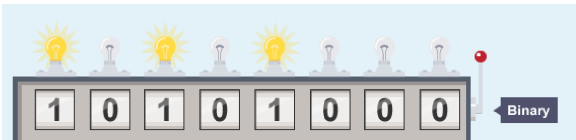
Fig 1.2. 1 Binary number 10101000 is represented as a sequence of 1s and 0s (on and off).
