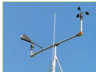
Figure 1.11 Wind Direction Indicator and Anemometer
