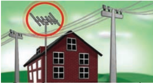
Do not fix antennas near current wires.
