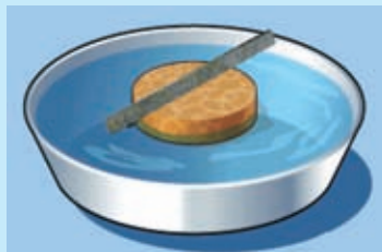
Figure 6.9 ▲ Considering the direction, that magnet turns, when it is floated on water using a piece of cork or styrofoam.
