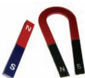
Figure 6.29 ▲ Permanent magnets made of steel
