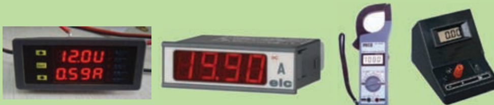
Modern voltmeters and ammeters assembled using digital technology
