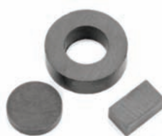
Figure 6.30 ▲ Permanent magnets made of ferrite
