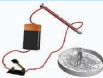
Figure 6.26 ▲ File clips fall off (do not attract) when electrical supply is disconnected
