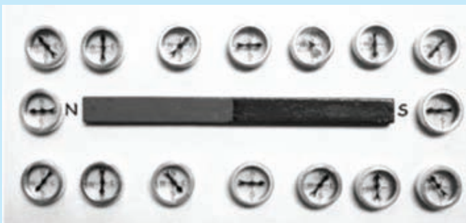
Figure 6.20 ▲ Positions of a compass needle around a bar magnet at various locations
