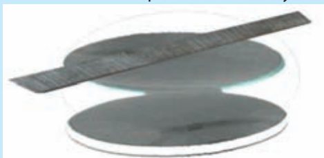
Figure 6.11 ▲ Observing the direction that the magnet turns when it is kept on a watch glass and moved freely on another watch glass
