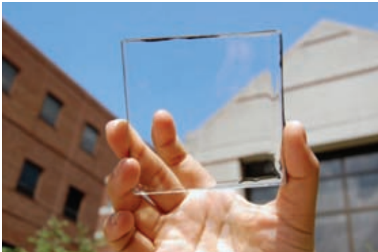
Transparent solar panels that can be used as house windows
