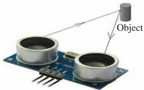
Figure 4.16 : How an ultrasonic sensor works
