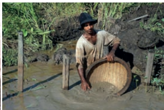
Figure 19.8(b) – Sifting of gems using a sifting pan
