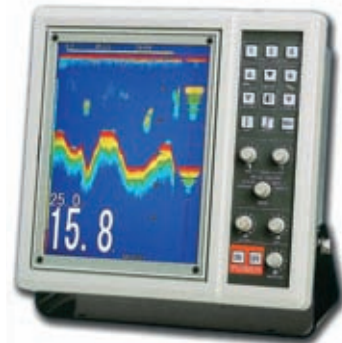
Figure 14.27 - How the information of ocean depth is depicted in an echo sounder
