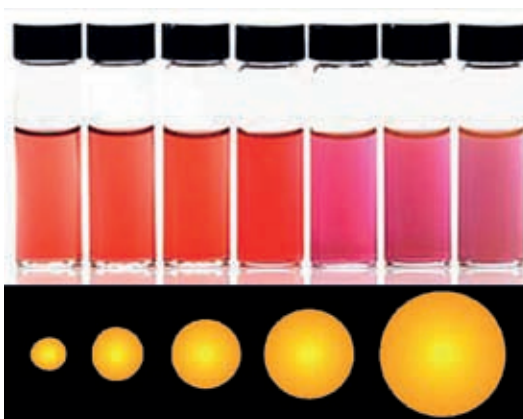
Figure 16.8 - Various colours are observed in gold nanoparticles when the size of particles are below 100 nm
