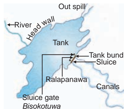
Figure 13.9 (b) – Major parts of a tank
