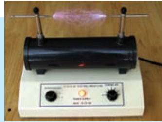
Figure 17.6 - Producing sparks by the induction coil
