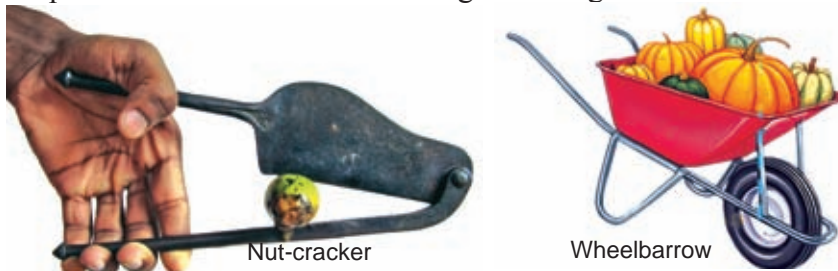
Figure 15.13 – Second order levers
