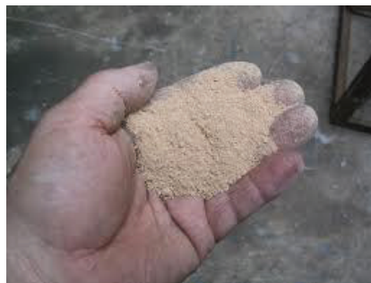
Figure 15.22 - Particulate matter of asbestos
