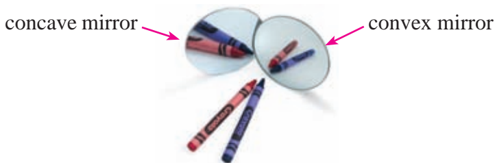
Figure 5.6 – Images formed by concave and convex mirrors
