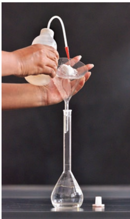
Figure 3.2.2 - Preparation of a standard solution
