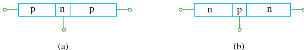
Figure 11.24 – (a) structure of pnp transistor (b) structure of npn transistor
