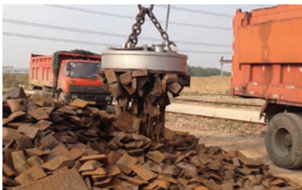
Figure 13.1 – Use of an electromagnet to remove scrap iron and steel
