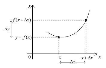
The corresponding change in y values denoted by  $\Delta y$  is equal to  $f(x + \Delta x) - f(x)$
