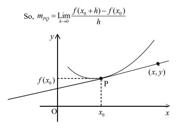
The equation of the tangent line at P to the curve y = f(x) is  $y - f(x_0) = m(x - x_0)$ .
