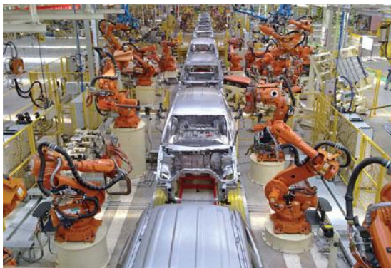
Fig 1.4.2 - Assembling car using computer-controlled robots
