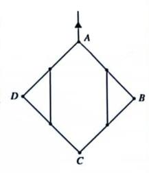
(b) The framework shown in the figure consists of five light rods AB, BC, CD, DA and DB smoothly jointed at their ends. It is given that AD = a,  $AB = \sqrt{3} a$ ,  $BAD = 90^{\circ}$ ,  $CBD = 90^{\circ}$  and  $BDC = 60^{\circ}$ . At each of the joints B and C, a load W is suspended and the framework is smoothly hinged at A to a fixed point and kept in equilibrium in a vertical plane with AB horizontal by a horizontal force B applied to it at the joint D.
