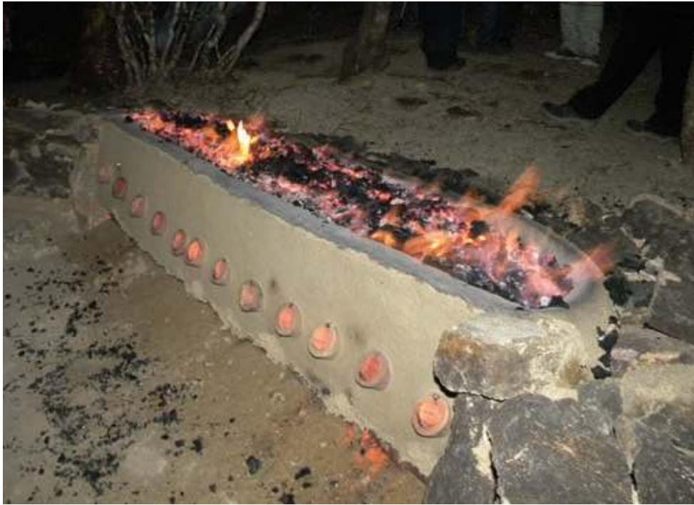
Fig:1.22 Furnaces used in extraction of iron
