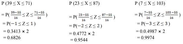
Thus, most of the characteristics that can be seen in a normal distribution can be seen in this frequency distribution. 100% of the observations in this distribution are located in the range of  $-3 \le Z \le +3$  from the mean.
